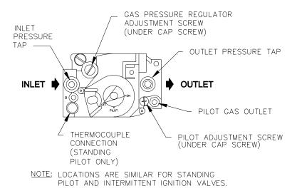
Figure 7.3: Valve Tapping and Adjustment Screw Locations
